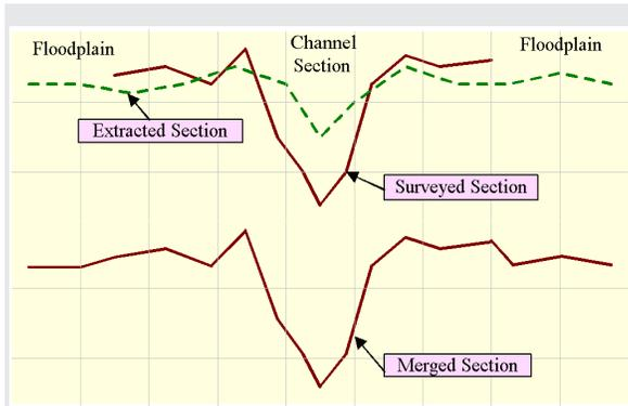
The TDMS combines surveyed and extracted cross-sections to provide a better extended channel cross-section representation.
