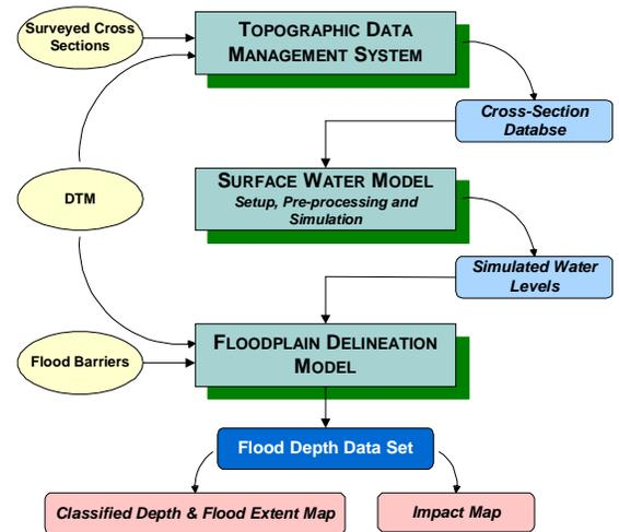
The Topographic Data Management System (TDMS) is capable of creating, editing and managing cross-section profiles stored in different formats. It also has the capability of extracting profiles from a DTM and merging with surveyed cross-sections. The cross-section database created by this system is easily accessible through an inter-
